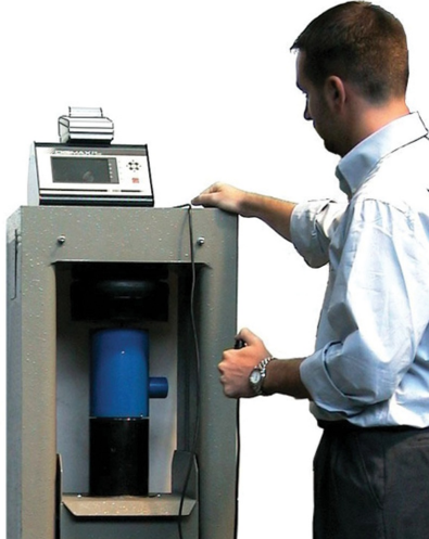
Load cell with Digital tester and printer during the calibration of a compression tester.
